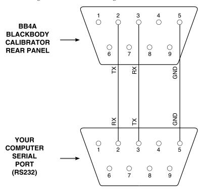
Figure 7. Connecting the BB-4A to a Computer's Serial Port
